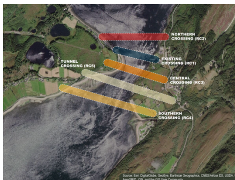
Images showing the 5 route corridors considered for a fixed link and a visualisation of one of the potential bridge options
