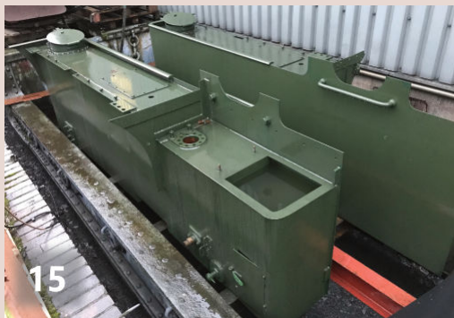
14: The bunker/cab components following removal and before dispatch to enable them to be copied and replaced, work that will be sub-contracted.
