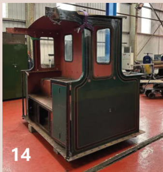
14: The bunker/cab components following removal and before dispatch to enable them to be copied and replaced, work that will be sub-contracted.
